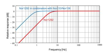
The frequency response may be corrected for use below the resonce frequency of  $4.5\ Hz$
