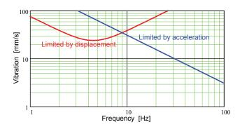
The lower limit is set by the noise floor in the transducer and measuring instrument. If the instrument has an electrical noise floor of 0,3  $\mu V$  – achievable for restricted frequency bands – this corresponds to a vibration level of 10-8 m/s or 0,00001 mm/s with the nominal sensitivity of 26 Vs/m. The noise in the transducer itself is even lower – mainly determined by the source resistance of 380 ohm which corresponds to about 0,04  $\mu V$  in a bandwidth of 250 Hz.
